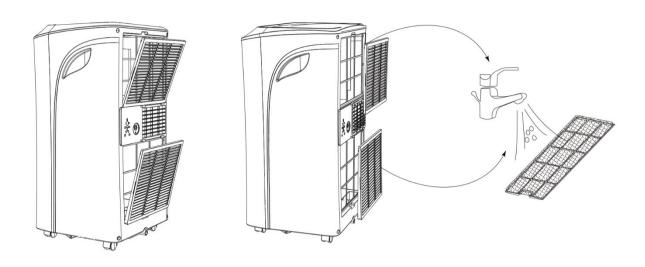
Before moving or storing the portable air conditioner, drain any collected water away using the drainage hose provided (see page 15 for further information). When storing the portable air conditioner use the cable compartment to store the mains cable. Clean the filters and then store the unit in its plastic bag or original box to protect the portable air conditioner from dust.
