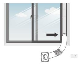
Step 5: Attach the duct via the air exhaust on the portable air conditioner using the duct machine adaptor.
