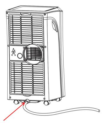
Securely attach the drainage hose to the outlet.
